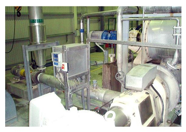
The Grubbens pump is due to its design suitable for use as a Booster pump directly after the Krima Disperser. The two units together form a unique solution for Medium Consistency (MC) discharge.
